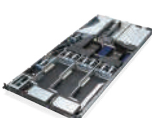
1U, 4GPU, 2TB DDR4, 8 NVMe Storage
